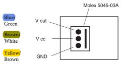
Fig. 7. Electrical connection C7195A2/B/C
