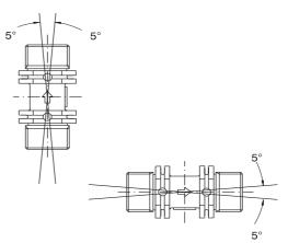
Fig. 6. Mounting position for C7195B
