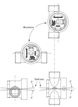
Fig. 4. Mounting positions C7195A2
