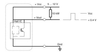
Fig. 8. Suggested interface schematic
