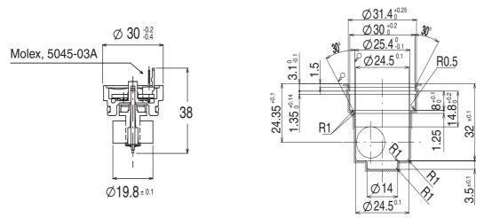
Fig. 11. Dimensional drawing cartridge (C7195C) and recommended seat dimensions for customzed body or water manifold
