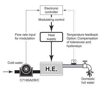
Fig. 1. Feed forward control loop concept
