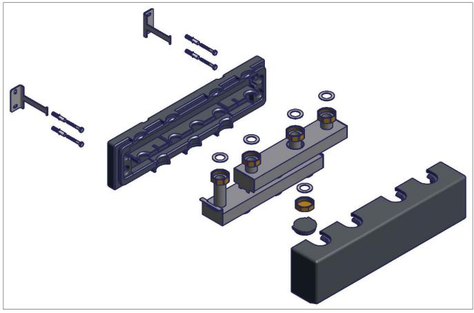
Fig. 2: Wall-mounted installation / optionally with wall bracket and fastening set
