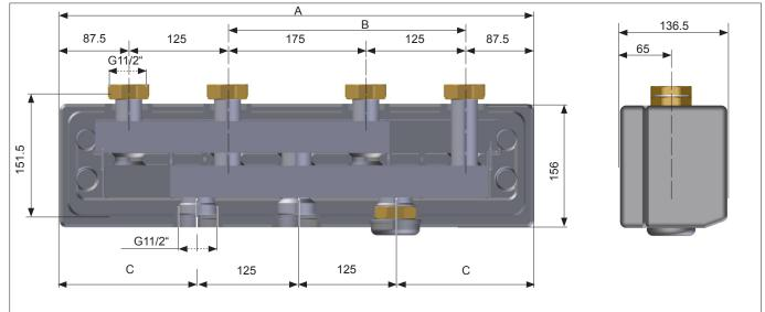
Fig. 1: Dimensions of 2-way boiler manifold; VB32-2 [mm]
