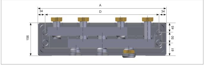
Fig. 3: Drilling dimensions of 2-way boiler manifold; VB32-2 [mm]
