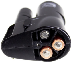
Fig. 15: Battery case, opened, with batteries
