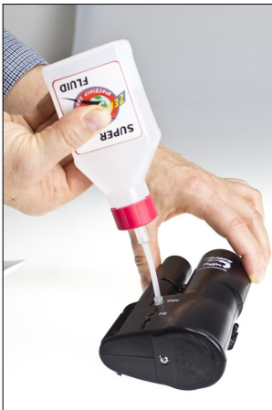
Fig. 19: Suction of the excess fluid
