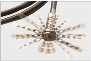
Fig. 5: Endpiece with chains driven by the drill
