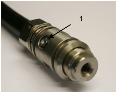
Fig. 6: Working end of the Rotary Viper with grease nipple
