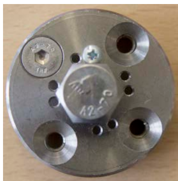
Fig. 8. End piece for holding chains with hexagon screw, secured by a security screw M3, 4 mm
