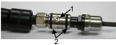
Fig. 7: Grease nipple at the drill end of the Rotary Viper; in the photo the grip is pushed aside.
