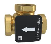
LK 822 ThermoBac is a 3-way check valve with low opening pressure and high fluid capacity. The valve is especially suitable for heating systems with storage tanks. The check valve prevents self-circulation from storage tank to boiler after the fire has gone out. In case of power failure or pump breakdown LK 822 ThermoBac automatically opens for self-circulation.
