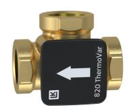
LK 820 ThermoVar® is a 3-way thermic loading valve for solid fuel/storage tank installations. The valve is intended to ensure both an optimal temperature stratification in the storage tank and a high return temperature to the boiler, thus incresasing the efficiency of the system. Tarring and condensation are prevented which prolongs boiler life. LK 820 can be equipped with an insulation - see under Accessories. For more information, please see the product sheet for insulations.
